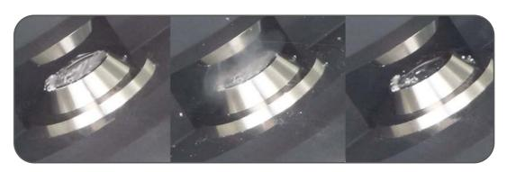
Cleaning effect of the WTW ultrasonic cleaning technology
