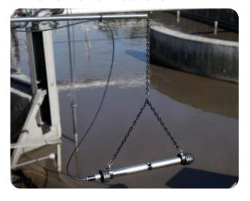
(Supplement kit Vis Set/EH in combination with swing mounting assembly EH/F 170-1,5)
